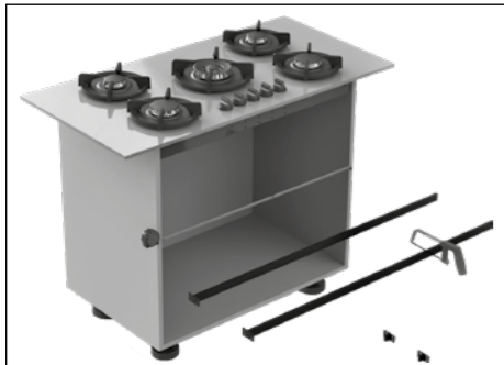
1. Determine the measurements of the cabinet and cut the support bar to size. ATTENTION: The proper length of the support bar = the interior dimension of the cabinet minus 4 mm.
